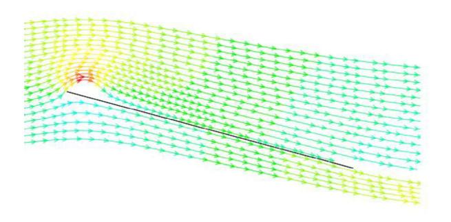
A (cambered) flat plate may be regarded as the simplest realization of a lifting device. During this thesis prediction (esp. those for the pressure around the trailing edge) of TDT should be compared with a carefully prepared CFD 2D setup [2] for laminar flow (RN < 100k). OpenFOAM is recommended as the code of choice.
