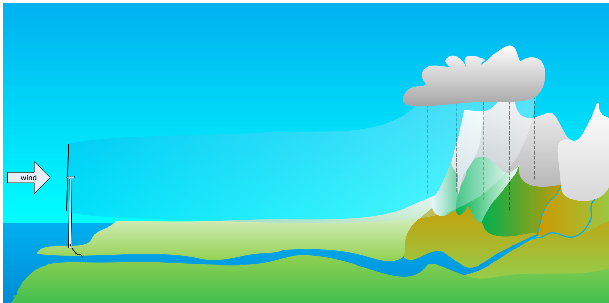
Figure 2 WT emits fresh water from a river. Onshore wind carries the vaporized water inland. Mountains deflect the humidified air vertically, which causes the air to cool down and the water to condense.
